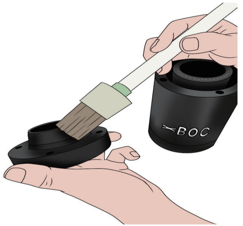
6. Lubricate the inner arc of the valve cover and the inner ring of the rubber hose
