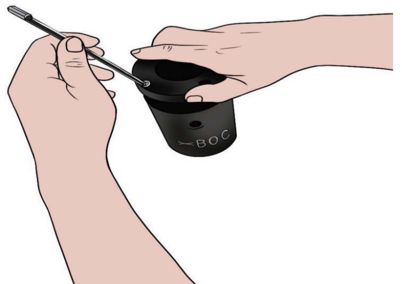
8. Fix the valve socket with screws, and tighten the screws cross-stitch.
