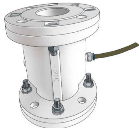
8. Finish assembly the flange , try to operate the valve at 3 bar several times then at 7 bar several times to watch the rubber form a lip seal and rebound normally.
