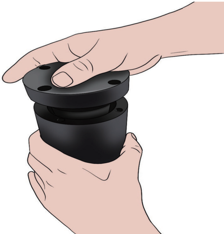
7. Screw the valve socket along the inner wall of the rubber hose, and then press the valve socket with one hand
